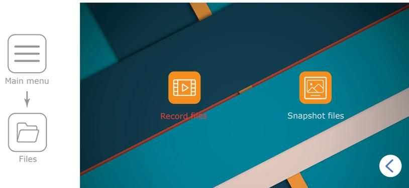
Press «Record files» or «Snapshot files» icon to enter snapshots or records playback menu then choose the file to play by moving joystick up or down. Press the joystick on the file to open side menu.
