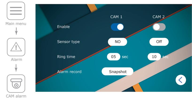
Software motion detector can observe and detect motion without any external sensors using any camera image changes with the time. Camera power that is used for motion detection should be constantly on to let the monitor observe image changes and detect it.
